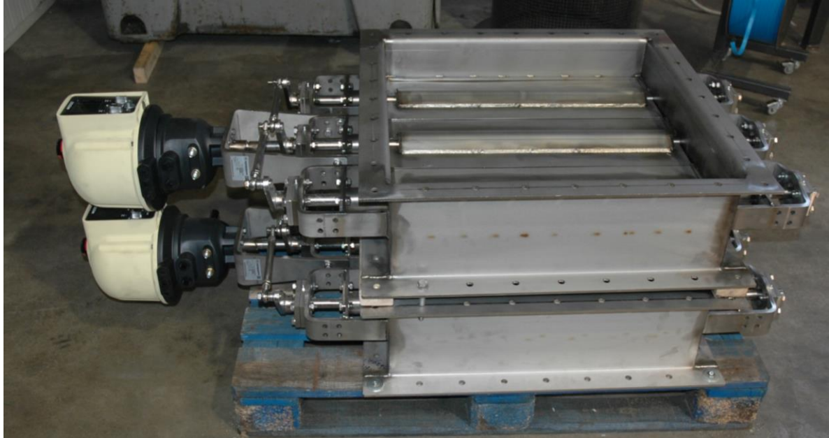
SERIES 64-LOUVRE VALVE 660 X 660 X 300 MM DESIGN TEMPERATURE : 700 °C MATERIAL: AISI 321 ACTUATOR: BERNARD CONTROLS AQ10 LOGIC READY FOR SHIPMENT TO AUSTRALIA
