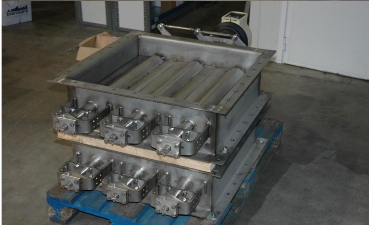
SERIES 64-LOUVRE VALVE 660 X 660 X 300 MM DESIGN TEMPERATURE : 700 °C MATERIAL: AISI 321 ACTUATOR: BERNARD CONTROLS AQ10 LOGIC READY FOR SHIPMENT TO AUSTRALIA
